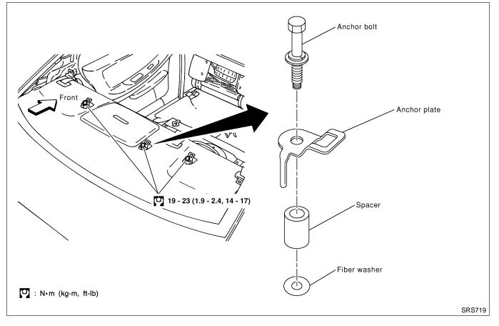
1. Remove tether anchor plate cover. Refer to BT-32, "SIDE AND FLOOR TRIM" for details.
