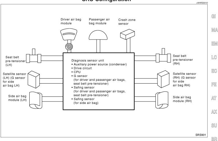
The air bag deploys if the diagnosis sensor unit activates while the ignition switch is in the "ON" or "START" position.
