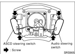
3. Remove steering switches from driver air bag module.
