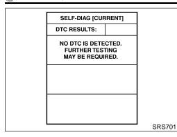
If no malfunction is detected on "SELF-DIAG [CURRENT]" even though malfunction is detected in "SRS Operation Check", check the battery voltage.
